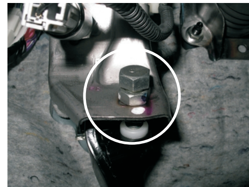
The pedal stop is measured and replaced by the enclosed clutch switch. The clutch switch must be placed on the same level as the pedal stop.
