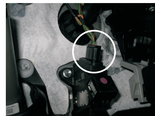
* Cut off the side guides from the connector on the pedal and the Plug'n Play harness. (Remove the pedal, for better access).
