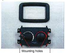
Attach the 4-pole and 2-pole plugs to the corresponding connections. Tighten the control element by fastening it with least 2 screws diagonally opposite to each other.
