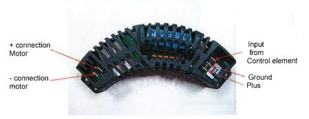
The supply cables to the motor must be as short as possible (10 cm). The module is not dirt or moisture resistant which ought to be taken into consideration when choosing its installation location.
