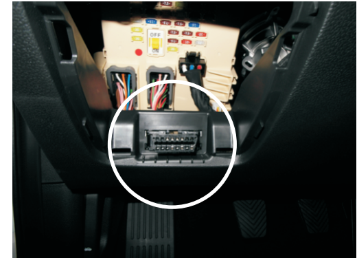
Dismount the original OBD connector from the bracket, and connect the enclosed Y cable. Mount the other end of the Y cable in the bracket.
