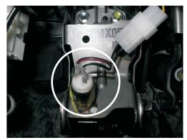
Remove the bolt and mount the enclosed clutch switch in the hole. The clutch switch must be placed on the same level as the pedal stop.
