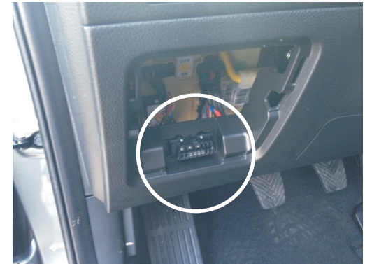
Dismount the originale OBD connecotor from the bracket, and connect the enclosed Y cable. Mount the other end of the Y cable in the bracket.
