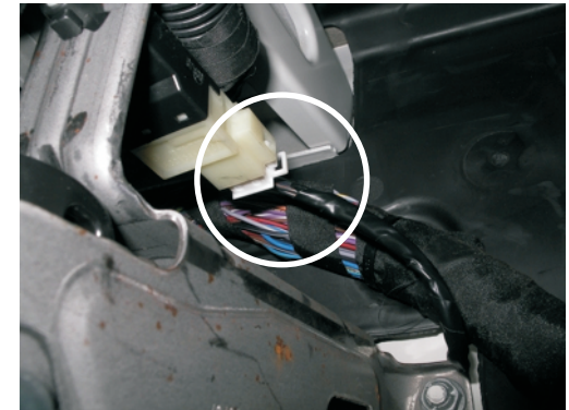
Ignition can alternative be found on ignition switch, black 6-pin connector, position 2, Black wire.
