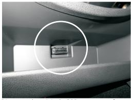
Dismount the originale OBD connecotor from the bracket, and connect the enclosed Y cable. Mount the other end of the Y cable in the bracket.
