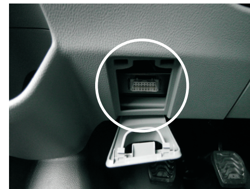
Dismount the originale OBD connector from the bracket, and connect the enclosed Y cable. Mount the other end of the Y cable in the bracket.
