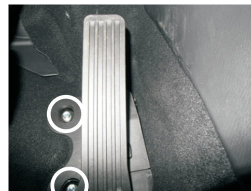
Dismount the accelerator pedal, by unscrew the two screws, for easier access to the connector.
