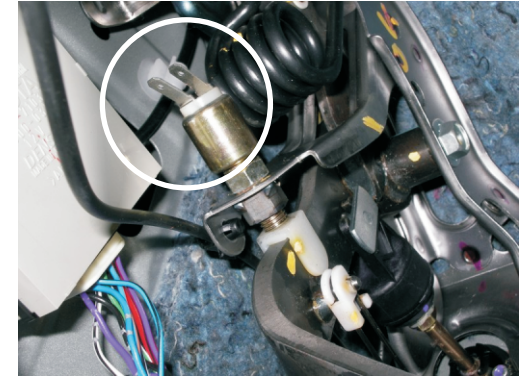
The Pedal stop is measured and replaced by the enclosed clutch switch. The clutch switch must be placed on the same level as the pedal stop
