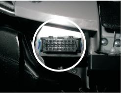
Dismount the originale OBD connector from the bracket, and connect the enclosed Y cable. Mount the other end of the Y cable in the bracket.
