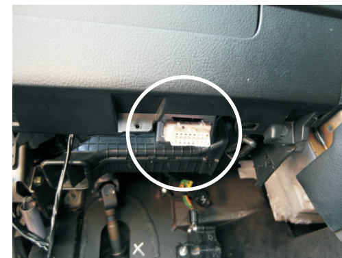
Dismount the original OBD connector from the bracket, and connect the enclosed Y cable. Mount the other end of the Y cable in the bracket.
