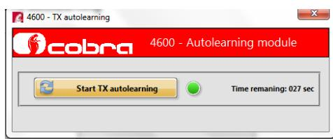
After having clicked "Yes" you have 30 s to auto-learning remote controls or driver cards. Press the button of the remote control or of the driver card after 5 s the led confirms with a flashing the successful store, press the button of the second remote control or driver card the led after 1 s confirms the successful store with a flashing. Continue with the same procedure to auto-learn other devices.
