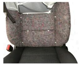
2. After removing the upholster, place the heating on a place, where it will be mounted and make holes in the seat, where the connection cables will be.
