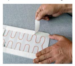
4. Stick the heating on the desired place and drag the connection cables through the holes in seat. Stick on each part of the heating so that it isn't crumpled and prevent damage. Don't place the heating in place, where the upholstering will be attached to the seat.
