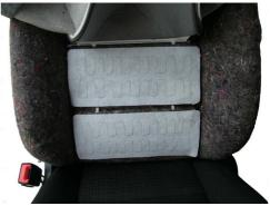
5. Put the upholster in original place and so the seat. Connect the cables from each part of the heating under the seat and fix them so they don't prevent moving the seat or damage.
