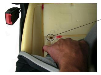
hole for power supply cables of the heating
