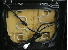
6. Connect the power supply cables according to the wiring diagram and place the other side of the cables under the seat in which the heating is installed. Place the cables so that you don't allow damage.
