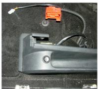
7. Place the control swith in a place chosen by customer. Common places are middle console, around the gear shift or near the seat. After choosing the right place, drill a hole with 20 mm diameter an mount the switch. Connect the switch to the cable harness.
