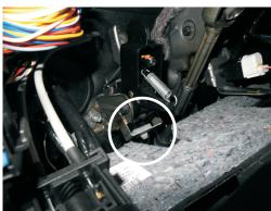
Remove the rubberplug, drill hole with a 10mm drill, and insert the enclosed clutch switch.
