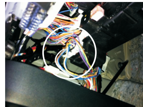
Alternatively, the CAN signals can be found behind Combi Meter in a white 24-pin connector. Green = CAN Hi - Pink = CAN Lo
