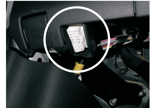
Dismount the originale OBD connectotor from the bracket, and connect the enclosed Y cable. Mount the other end of the Y cable in the bracket.
