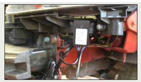
Once the lights have been connected up in the vehicle, the two control units for the daytime running lights have to be fixed in the engine compartment. Then the control unit cables can be routed to the daytime running lights.
