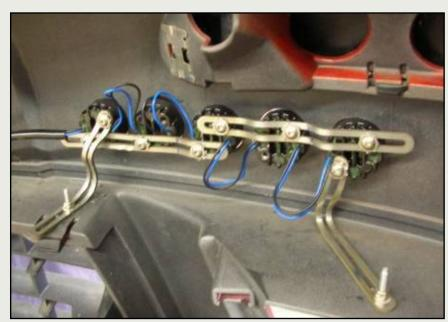
Once the holes are the right size (3 cm diameter) and the modules the right distance apart (1-15 mm), the daytime running light can be inserted and fastened to the front apron. In this case, the stainless steel brackets were used again for mounting.
