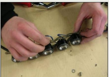
In this case, stainless steel rails were used to fasten the individual modules in place.
