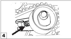
Fit the new timing belt and install the engine mounting/bracket.
