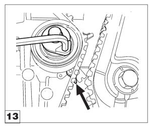
Use an allen key to turn the tensioner **anti-clockwise** to apply tension to the belt.
