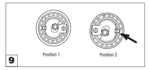
When fitting a new belt the automatic tensioner must be in **Position 1**. Fit belt and then turn tensioner **anti-clockwise** until pointer is in **Position 2**.
