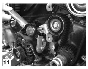
Fit torque wrench and 8mm hexagon socket bit to tensioner lever arm and apply 25Nm. torque in a **clockwise** direction.
