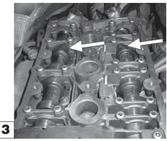
Turn the crankshaft **clockwise**, using the centre bolt of the crankshaft, so that the lobes of the inlet and exhaust camshafts for No. 3 cylinder are angled upwards, (Left-hand bank, when looking from the camshaft sprockets).
