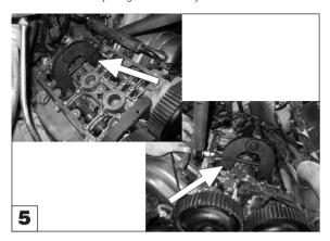
Fit one of the AST4941 Camshaft Setting Plates to the camshafts at No. 3 cylinder postion on the left-hand bank (when looking from the camshaft sprockets), and the other Setting Plate onto the camshafts at No. 4 cylinder position right-hand bank (when looking from the camshaft sprockets).
