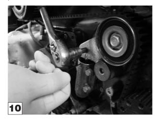
Apply pressure to the lever arm in an **anti-clockwise** direction until AST4593-1E Locking Pin can be removed. Remove the Pin to release the tensioner plunger.
