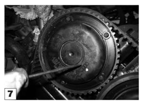
Prise off the circlips and blanking plugs of all four camshaft sprockets, and slacken each camshaft sprocket bolt, leaving the bolt in place.
