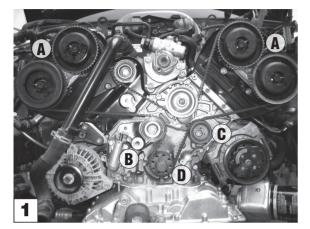
The VAG 3.0 V6 petrol engines are 'Quad Cam' engines with the timing belt directly driving all four camshafts from the crankshaft.
