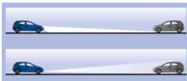
Fig.: System comparison of low-beam lights to daytime running lights
